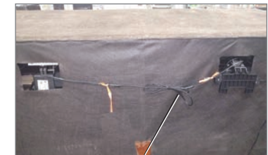
Wind and Secure Excess Y-Cable with Cable Tie (Applies to Sofa and Loveseat Styles)
