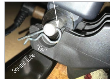
Arrow Shows “Ear” Stopping on Motor Pin
